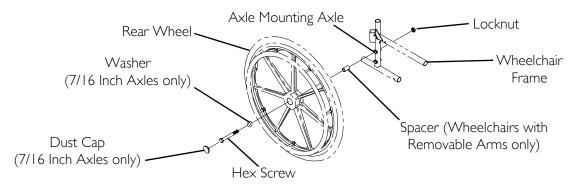
FIGURE 7.1 Removing/Installing Rear Wheels
